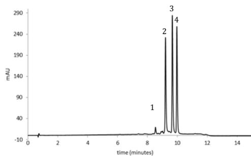
Fig 9: Separation of a mixture of compounds 1, 2, 3 and 4 on C18+ phase with t-MeAmOH additive
