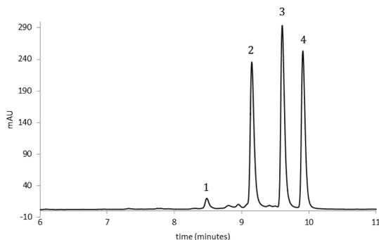
Fig 8: Separation of a mixture of compounds 1, 2, 3 and 4 on C18+ phase without t-MeAmOH additive (exploded view)
