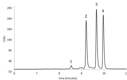
Fig 10: Separation of a mixture of compounds 1, 2, 3 and 4 on C18+ phase with t-MeAmOH additive (exploded view)
